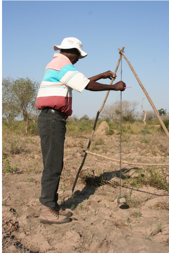
Figure 1: Silva Chauque has been using the 'A' frame for water harvesting to help improve his crops. He lives in Tchalefu in the Chigubo District, Mozambique. Photo: Practical Action | Emma Judge
