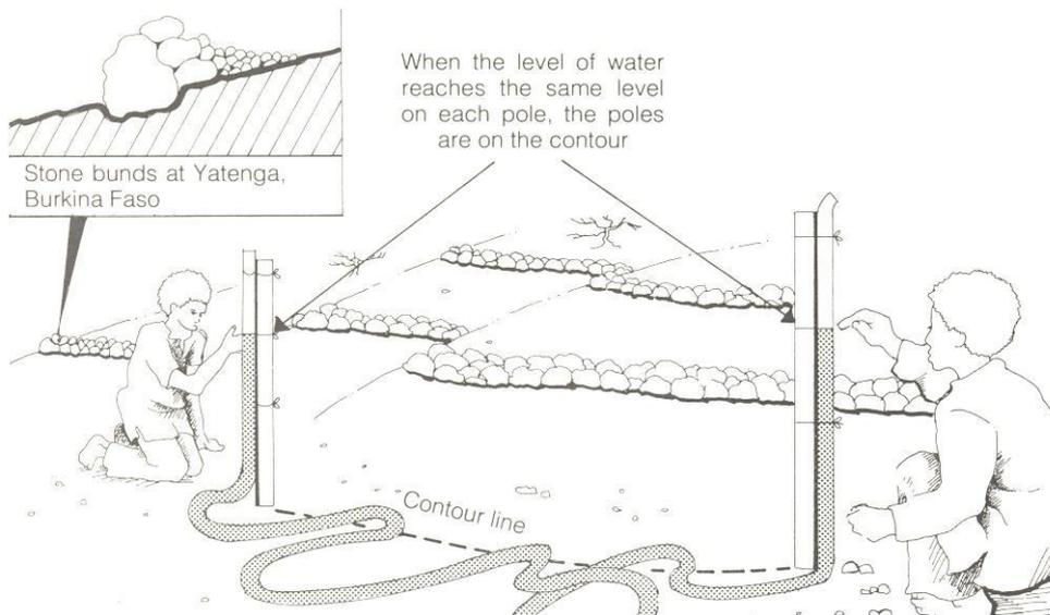
Figure 3: Finding the contour line using a water level, and building a stone bund.
