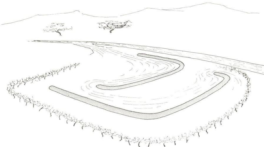
Figure 1: The caag system, showing the live thorn fence surrounding the earth bunds.
