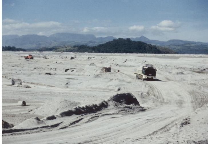
Figure 1: Volcanic ash in Indonesia being gathered for use as a pozzolana. Photo: Practical Action (not a Practical Action project)
