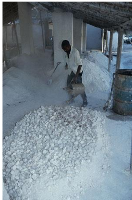
Figure 1: Slaking. Hydrated lime is produced by adding water to quicklime. Chenkumbe Hills Area, Malawi. Photo: Practical Action / David Mather.
