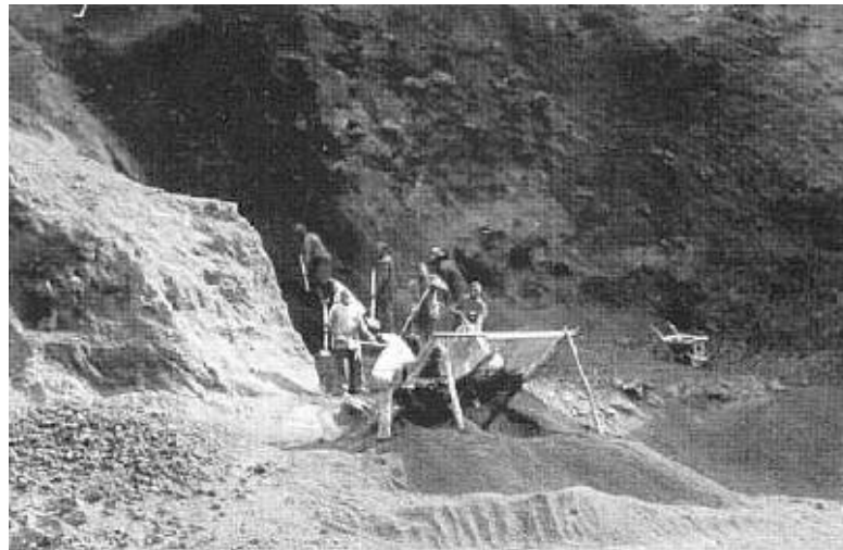
Figure 2: Volcanic ash pozzolana being excavated, Rwanda.
