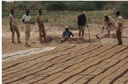
Figure 2: Slop-moulding and drying of bricks. Photo: Practical Action
