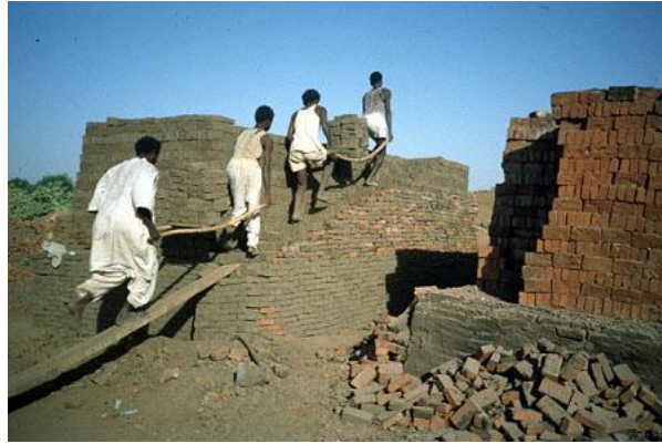
Figure 3: Staking of bricks for clamp-firing. Photo: Practical Action
