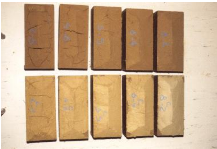
Figure 3: Test carried out on unstabilised and stabilised mortars to determine the optimum soil/sand ratio. Photo: CRATerre/EAG
