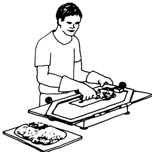
Figure 2: Work the mortar mix under vibration
