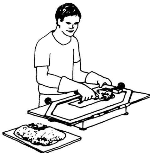
Figure 3: Smooth under vibration
