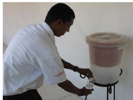
Figure 1: Diagram and picture of Clay Water Filter. Source: Practical Action Technical Brief – Clay Water Filters
