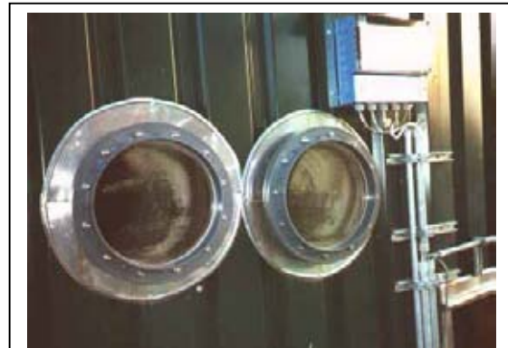
Figure 11: Control glasses for an industrial digester for solid organic waste, TBW, Germany
