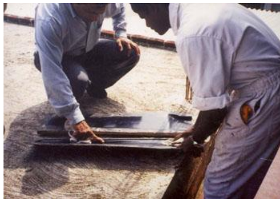
Figure 4 : Mr. W.A. Fernando of the Dinusha Marine Works in Panadura manufacturing blades for small wind systems. Photo: Practical Action South Asia.
