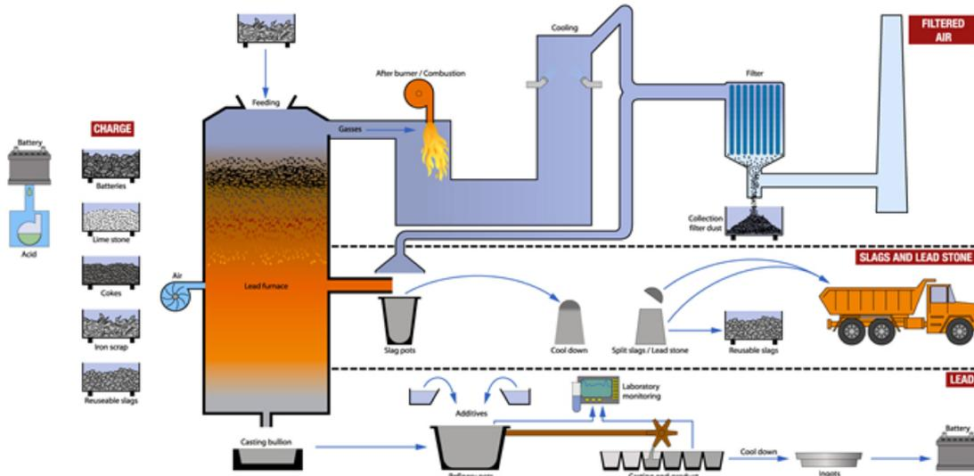
Figure 2: schematic drawing of the recycling process of lead acid batteries (source: [www.campine.be](http://www.campine.be))
