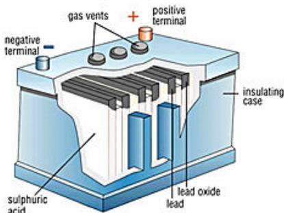
Figure 1: Example of a lead acid battery
