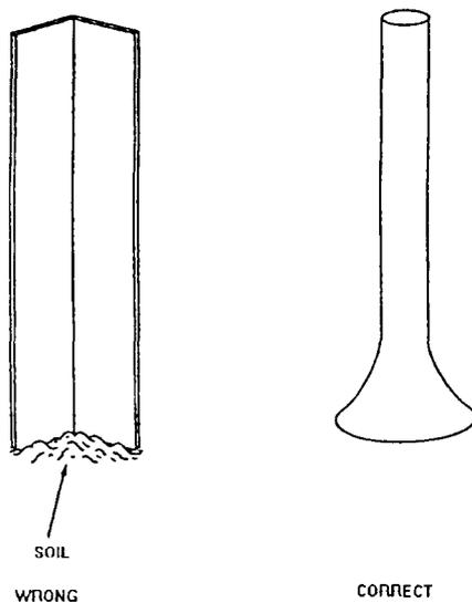
Figure 1: Support leg design to prevent soil accumulating
