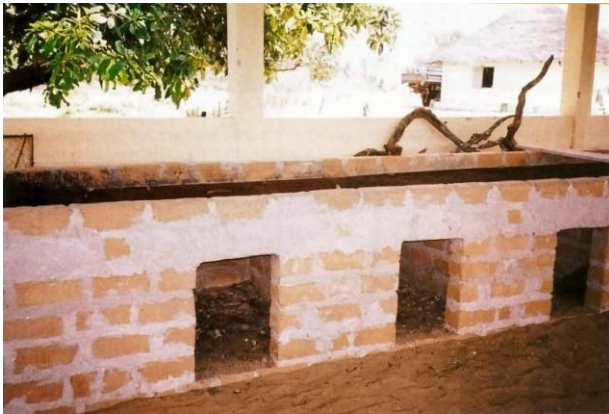
Figure 3: Improved Chorkor smoker. Photo: from Jallow, 1994.
