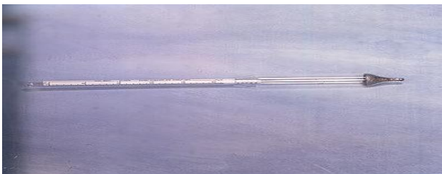
Figure 1: A salt hydrometer to measure the strength of salt in brine. Photo: Pete Fellows
