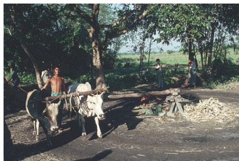
Figure 1: Animal powered crusher. Photo: Neil Cooper/Practical Action.
