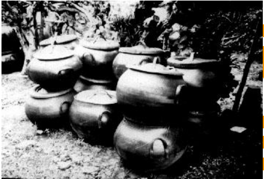
Figure 4: Garbage containers made from Truck tyres. Manila, The Philippines.
