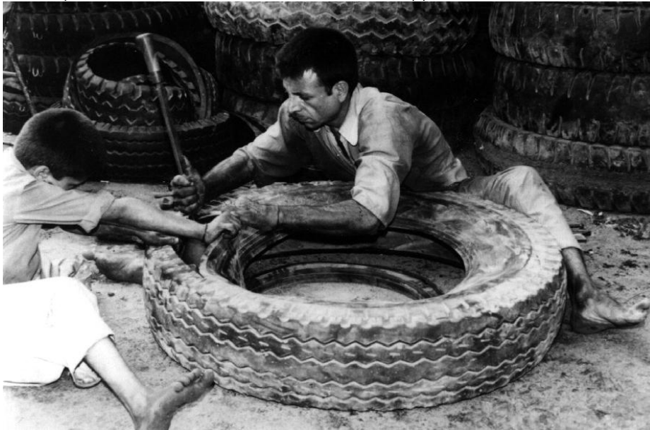
Figure 2: Manual Separation of the Tread from the Sidewalls, Karachi, Pakistan Photo: PCSIR – WASTE
