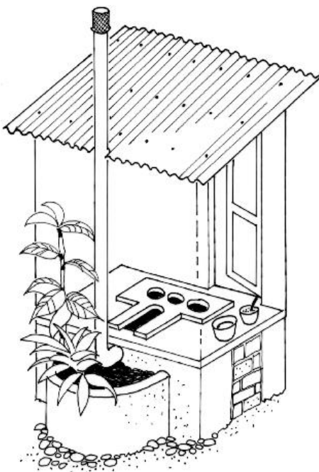
Figure 3: Kerala double vault dehydration toilet [Illustrator: Hans Mårtensson; Source: Winblad and Simpson-Hébert, 2004]
