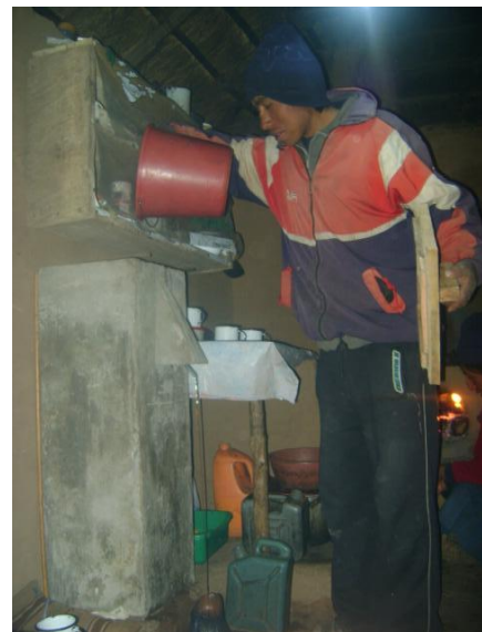
Figure 2: A domestic bio-sand water filter being used in Peru. Photo: Soluciones Prácticas.
